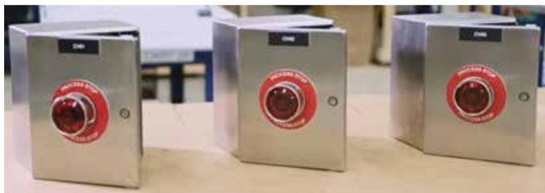
The Steinhauer precisely drilled holes in the enclosures (top), allowing a Panel Shop wireman to install the push buttons (bottom).
